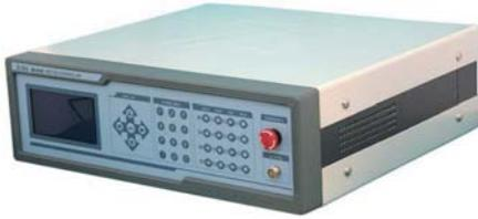
MC600 series products are high-performance controllers designed and manufactured by Zolix. They employ 32-bit DSPs to realize 3-axis linear interpolation and 2-axis circle interpolation with closed-cycle feedback with each axis. They can be operated with a built-in SD cards which means that host computer is not a necessary part in the controlling systems.
