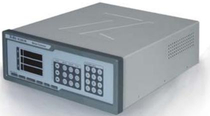
SC series products are motorized stage controllers for 1-3 axis point-to-point integrated position controlling. Stepping motor controlling cards are built-in and display panel is also provided. RS232 and USB ports are standard (not be used at same time) and can controlled with Zolix Motion Manager software. If customer requires, communication protocol or OCX controls can be provided.
