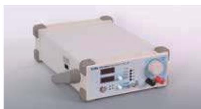
Xe arc lamp light sources are the preferred artificial sources to simulate sunlight. The high color temperature (6000K) of the Xenon lamps is a close match to the solar temperature. This results in very similar solar spectra in the UV and VIS although the source has some Xe emissions lines in the near IR.
