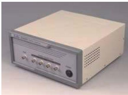
DCS210PC single photon counter, in photon counting function it based on the realization chopper control function phosphorescence and fluorescence lifetime testing. The instrument is also equipped with 3DC voltage input analog signal acquisition channel (16Bits, 0~10V) and 1 analog signal output channels (12Bits, 0~10V), convenient combination system.
