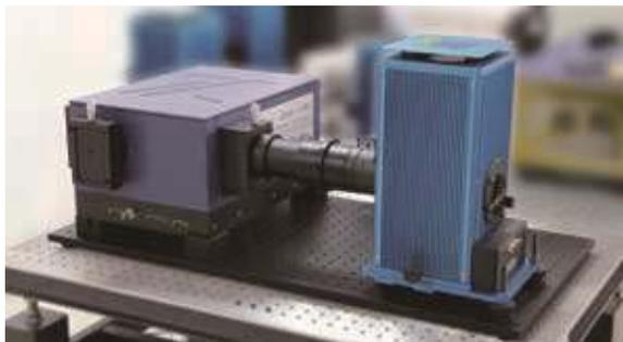
The Tunable Light Source (TLS) are pre-aligned, pre-assembled illumination systems capable of outputting monochromatic light from 200nm. This is a complete plug and play system and includes TLS-C1 software.
